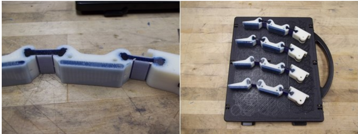
Fig. 6 – Minimal cuts required to remove the mold cavity walls
