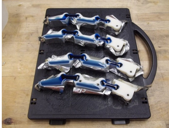
Fig. 5 – Enough mold material poured such that urethane just barely overflows
