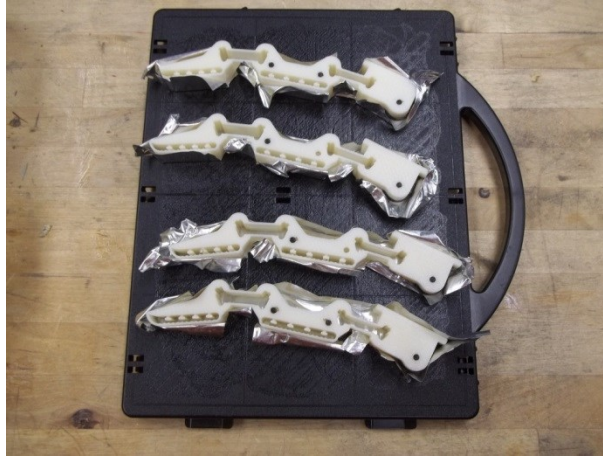
Fig. 3 – 3D printed finger frame sealed on bottom face with adhesive
